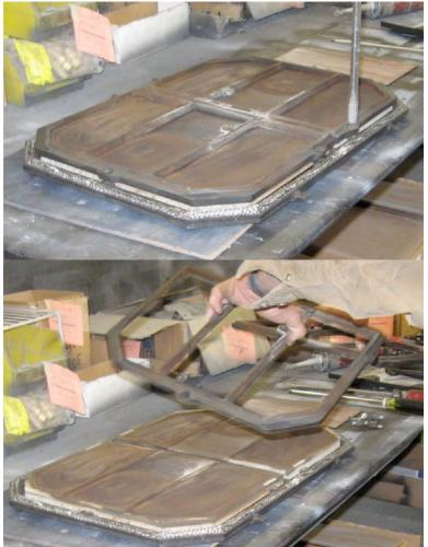
6. Remove the stone(s) to be replaced. Push the stone(s) up and out of the frame from below.
