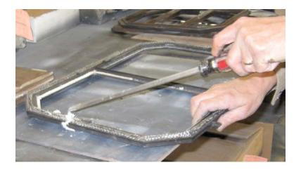
8. Dry fit a length of gasket in the frame. Trim to fit. Apply a small bead of gasket glue to the frame and install the pre cut length of gasket. Do not allow the glue to dry before the gasket is in place or it will become hard and lumpy.
