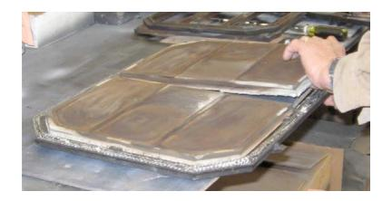
7. Remove the gasket that rests under the stone(s). Use a putty knife or flat blade screwdriver to clean the residue from the frame as much as possible.
