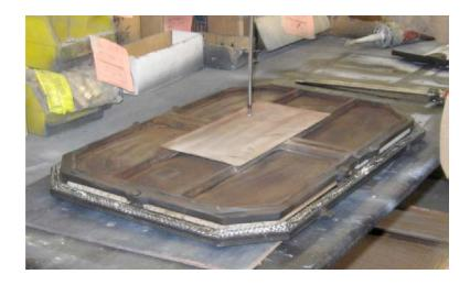
5. Use a large flat blade screwdriver to remove the six screws from the two cast stone retainers.
