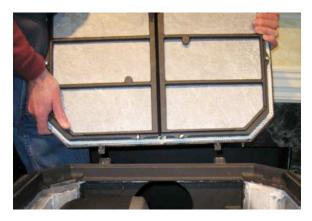
3. Place the top lid upside down on a workbench with a piece of cardboard underneath it to protect the bench and the lid. It is helpful to elevate the front edge of the lid with a block of wood.
