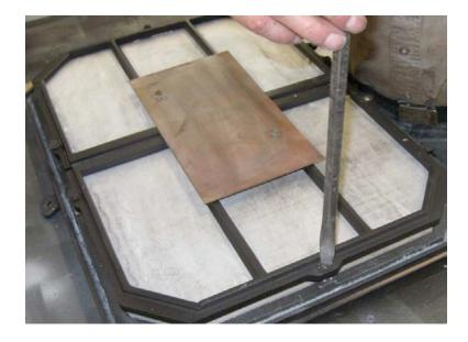
13. Replace the heat shield on the stone retainers if you have one.
